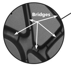
FMVSS -119 Section (c) and The Federal Motor Carrier Safety Regulation Part 393.75 state that (non – steer axle) "tires shall have a tread groove pattern depth of at least 2/32nds of an inch when measured in a major tread groove. The measurement shall not be made where tie bars, humps or fillets are located."
