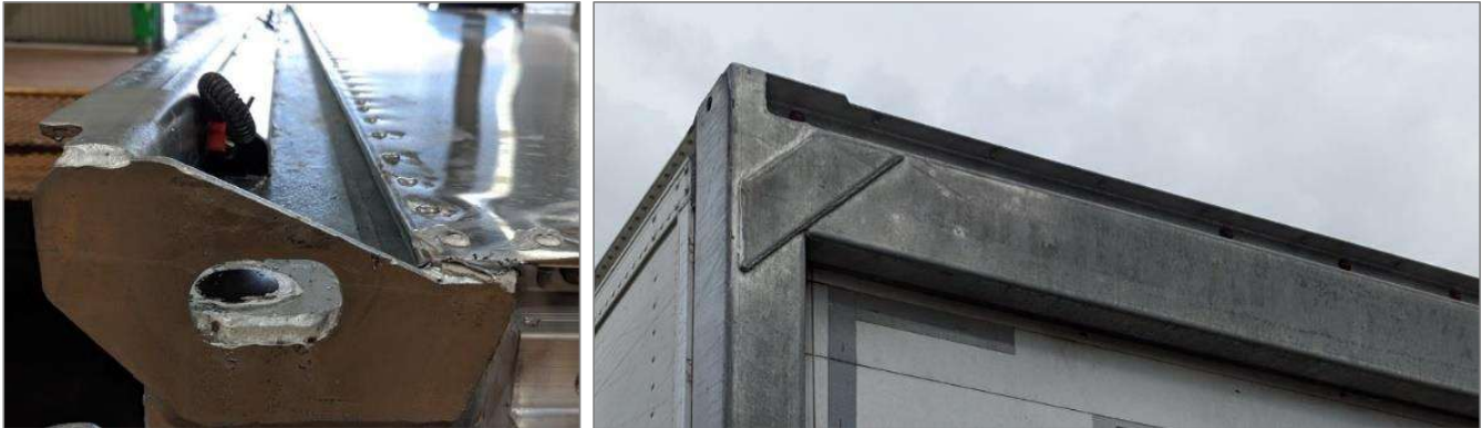
Figure 5: Extended Rear Flange Trailer Photographs
