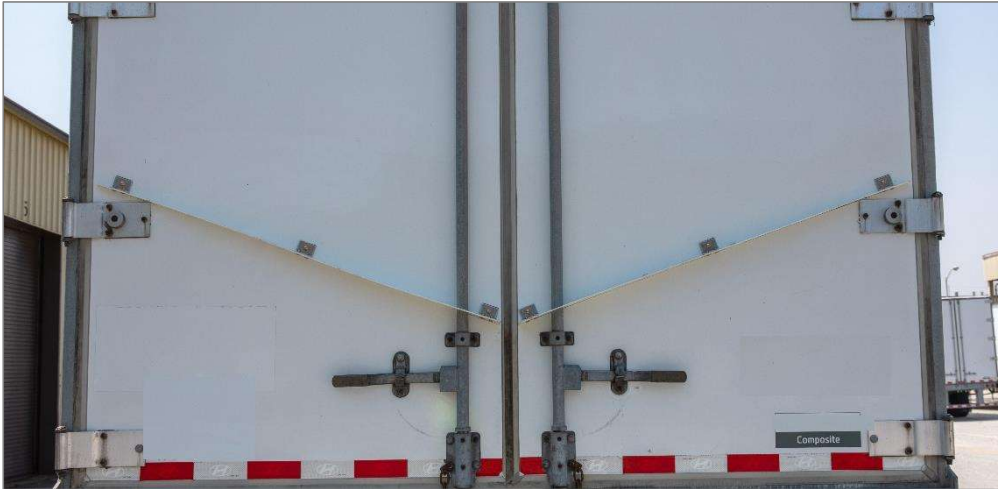
Figure 8: Wake Reducer Installations on Swing Doors
