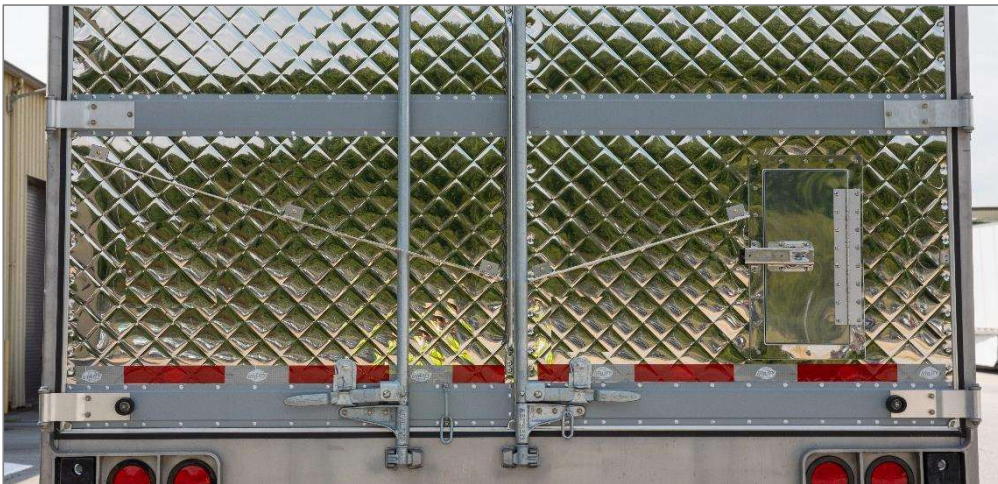
Figure 9: Wake Reducer Installation on a Roll-up Door
