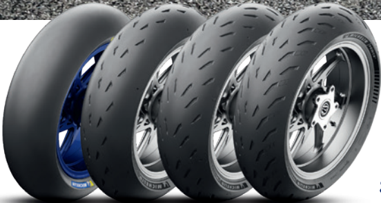
From left to right, MICHELIN Power Slick (MotoGP™ winner), MICHELIN Power Cup2, MICHELIN Power GP, MICHELIN Power5
