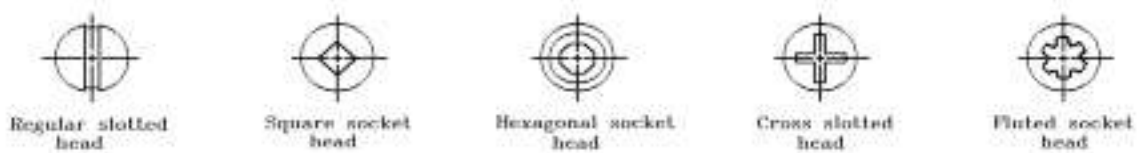
Figure 1-14 Different types of screw head slots
