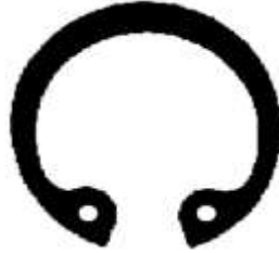
Figure 2-15 Typical snap ring
