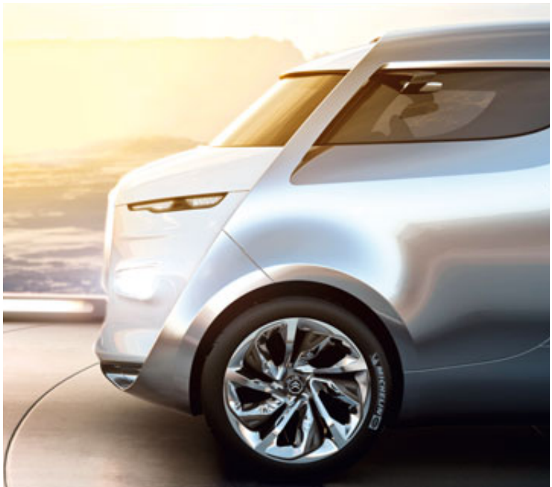
The Citroën Tubik concept car is equipped with a narrow 22-inch Michelin prototype tire.
