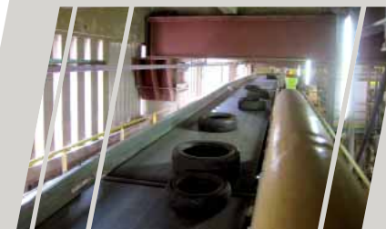
▲ Burning whole end-of-life tires in a cement plant furnace.
