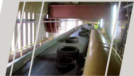
▲ Burning whole end-of-life tires in a cement plant furnace.
