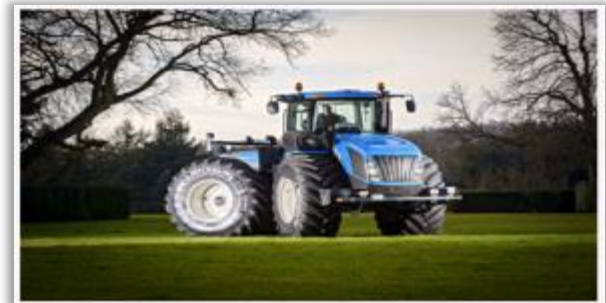
MICHELIN AxioBib IF 850/75 R42: loading capacity of 9,5 tonnes at low pressure
