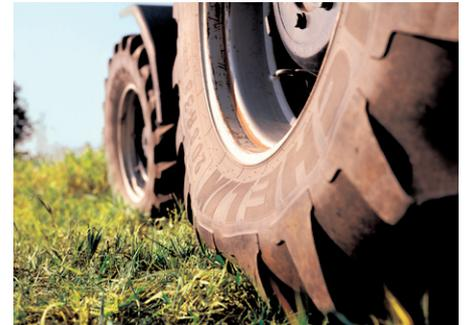
Thanks to MICHELIN UltraFlex Technologies, **the tyre footprint increases by 20% for the same weight and dimension\*.** This means that the soil is less compacted and thus better preserved.
