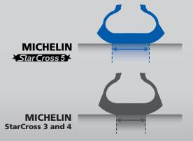
This combination of the new casing, engineered to optimise the size contact patch, and aggressive front and rear tread patterns, specific to the type of usage and terrain, offer maximum levels of grip for precise steering and traction even when racing in very difficult conditions.
