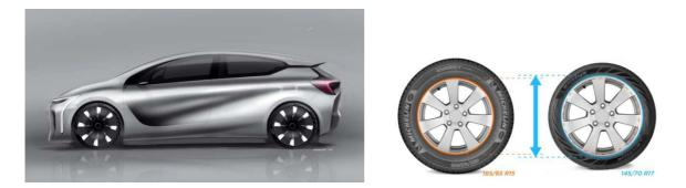
Michelin engineers designed an entirely new-sized tire (145/70 R 17) specifically for this concept car to provide it with outstanding aerodynamic qualities and energy efficiency.
