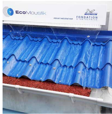
Installation of the AGLOSTIC® in the gutters
