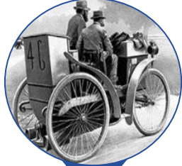
Éclair, the first car with pneumatic tires
