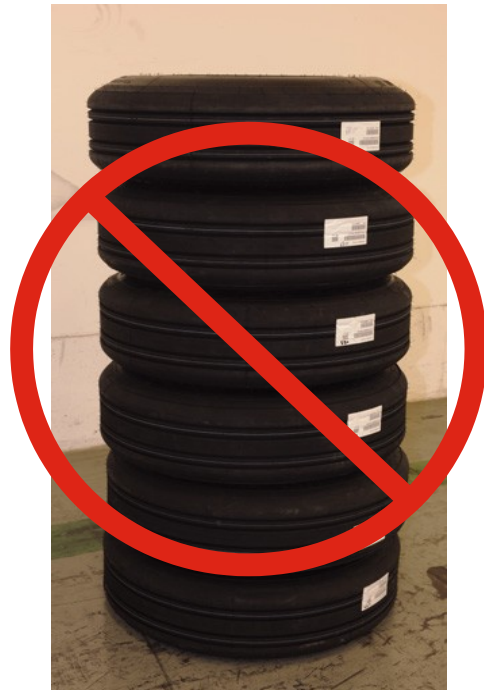
Figure 305. Store Tires Vertically in Racks (Left). Tires Stacked Horizontally (Too many tires) (Right)
