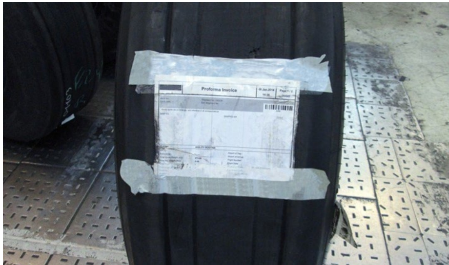
Figure 549. Recommended Placement of Adhesive Labels on Tires
