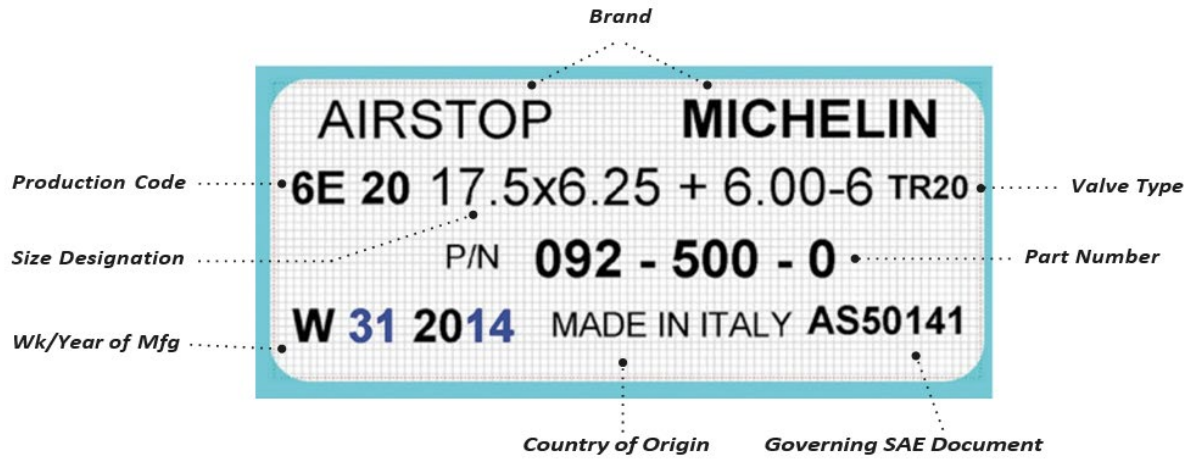
Figure 207. Typical Aircraft Tube Markings
