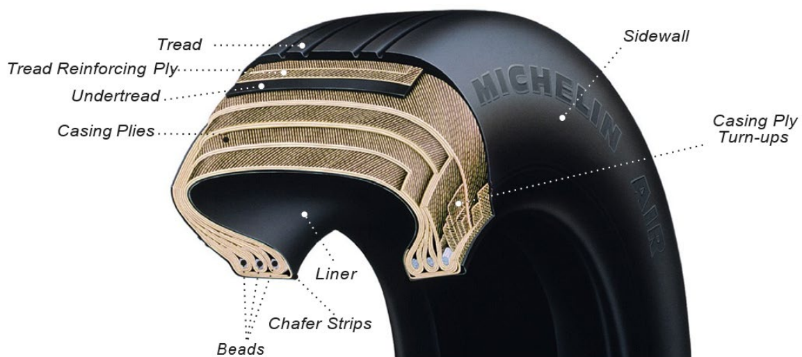
Figure 103. Bias Aircraft Tire
