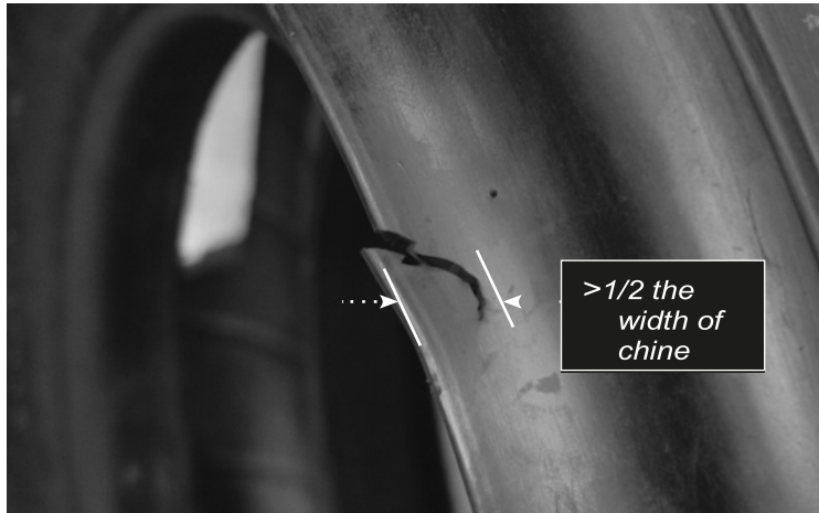
Figure 538. Damage to Chine Tire
