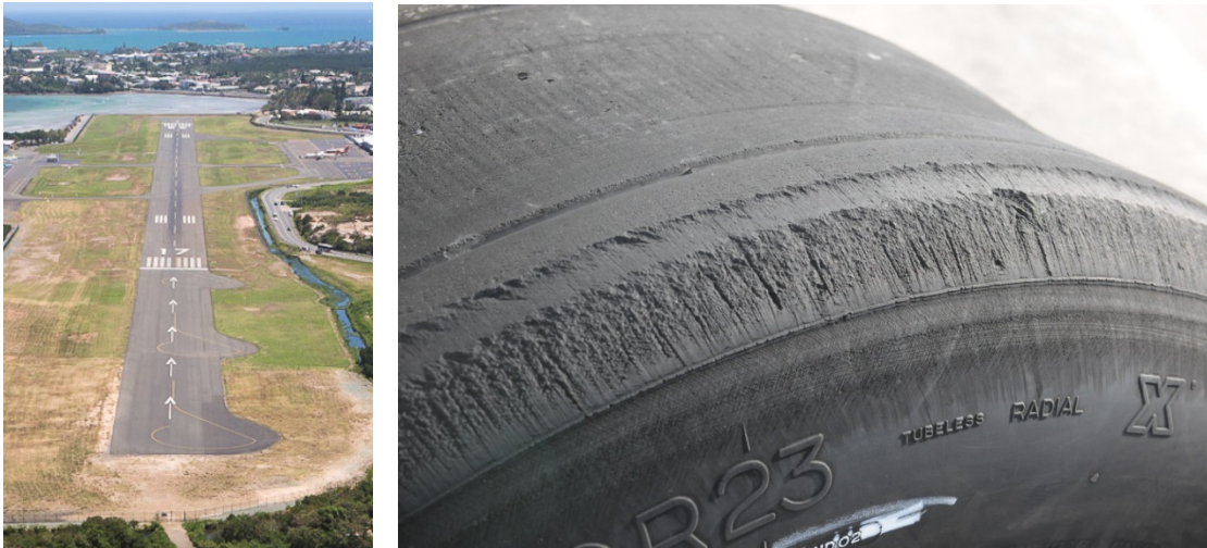
Figure 543. Lateral shoulder scratches from pivot turns
