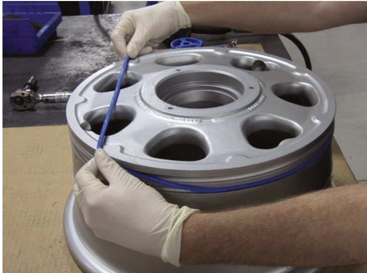
Figure 404. Installation of O-Ring on Inner Wheel Half
