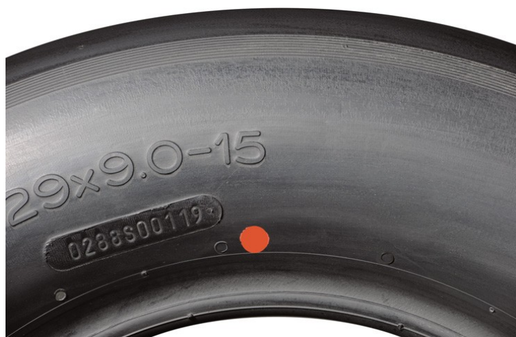
Figure 405. Tire's Red Balance Mark
