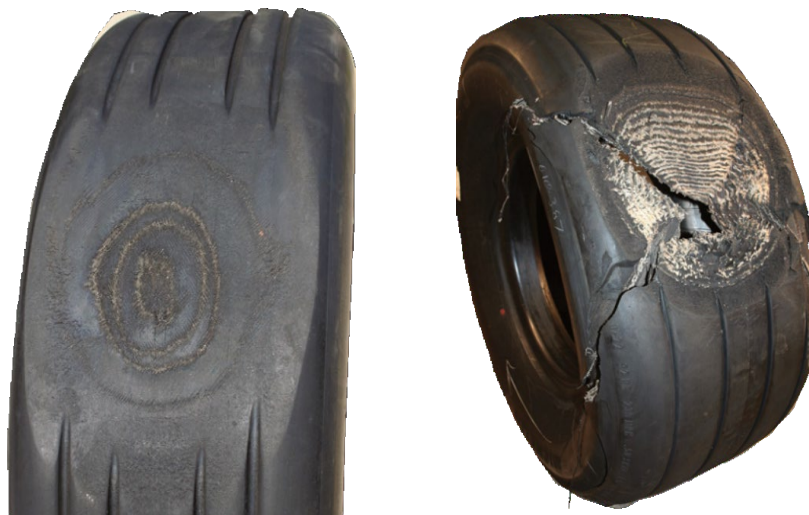
Exposed Reinforcing Plies
