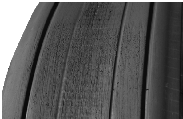
Figure 524. Aggressive Wear from Heavy Braking
