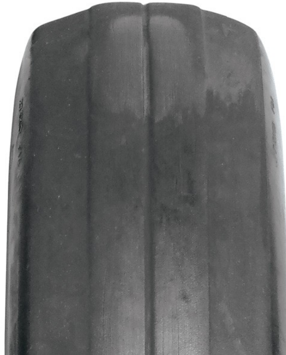
Figure 514. Shoulder Wear due to Underinflation
