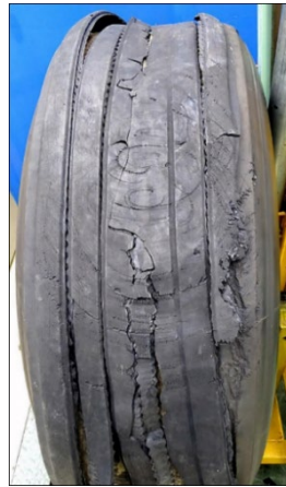
Figure 533. Tread detached due to lateral scrubbing
