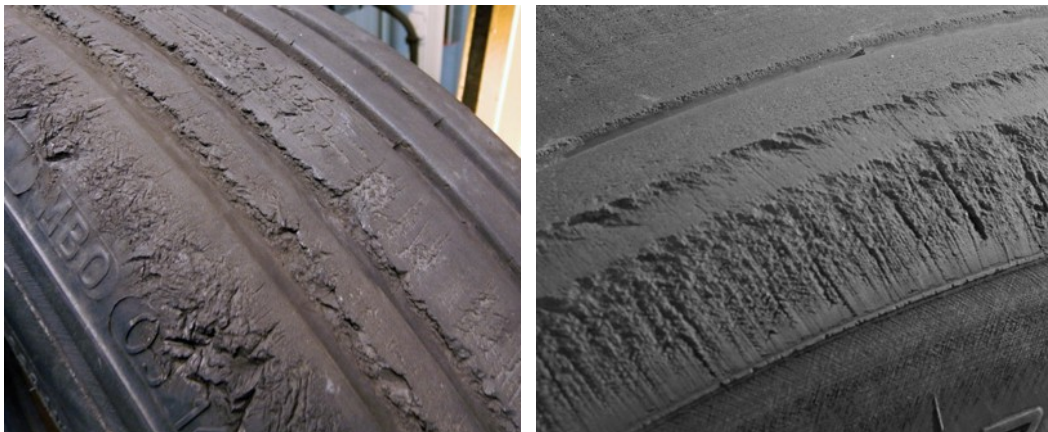
Figure 544. Lateral Scuffing, High Speed Turns, Pivot Turns
